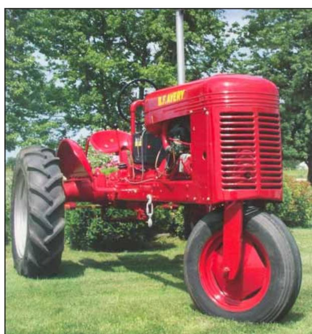
vious. The tractor has no foot pedals for the brakes. Levers on each side of the seat allow the operator to apply the brakes on either rear wheel individually and lock them in place.
